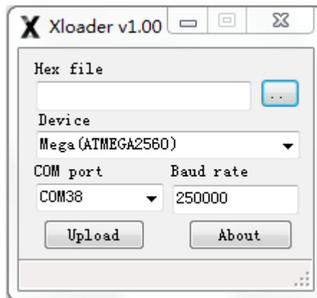
3. Set according to the picture. Select firmware file. Select the correct COM port.
